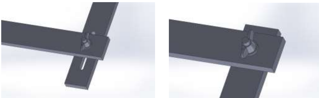
Detail of the slotted connection at one end and hole-to-hole connection at the other
