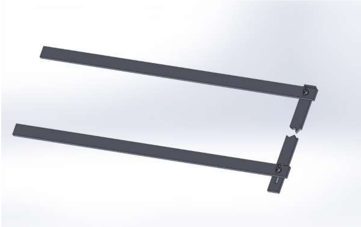
The assembled gauge showing the horizontal bar and two hinged pieces.
